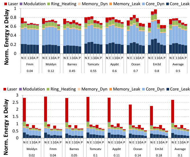
FIGURE 28: Energy x Delay Product in radix-16 (top) and radix-64 (bottom) MWSR crossbar. The evaluated designs are from left to right: No-Ctrl (N), Power_Eq (E), Static-1 (1), Static-10 (10), Adaptive (A), and Perfect (P).
