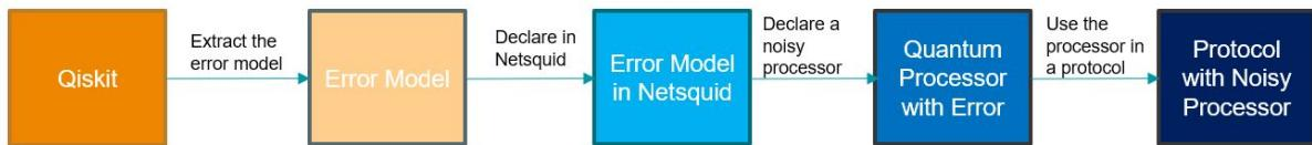
Step 1: Extract out the error model of a given backend in Qiskit.
