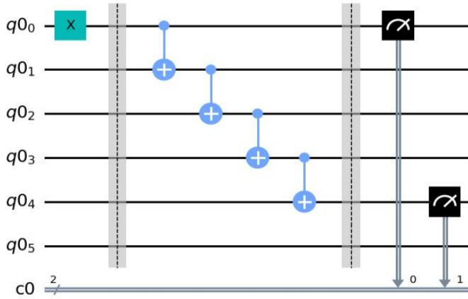
The figure shows the schematic of the CNOT chain circuit. Qubit  $q_{0_0}$  is initialized in the  $|1\rangle$  state and a series of CNOT gates are performed as shown. In the end, qubits  $q_{0_0}$  and  $q_{0_4}$  are measured. This process is repeated 1000 times and the average rate of success ( $q_{0_0}, q_{0_4}$  measurement outcome 11) is recorded for both Qiskit and NetSquid.
