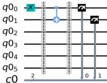
The figure shows the schematic of the circuit. Qubit  $q_{0_0}$  is initialized in the  $|1\rangle$  state and a CNOT is performed between  $q_{0_0}$  and  $q_{0_1}$ . After that, the two qubits are measured, and the results of the measurements are recorded. This entire process is repeated 1000 times and the results are aggregated. A successful run results in measuring 11. Due to errors in the noisy quantum processor, other results will also be recorded with some probability.
